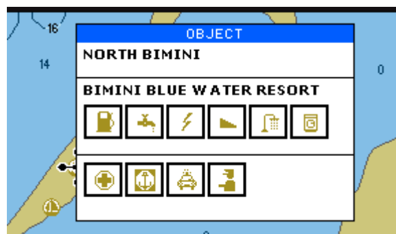
Sample filling station, service marks
