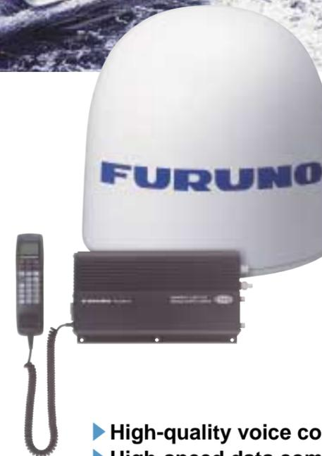
FELCOM 50 offers almost the same services as Fleet F77 within the coverage of spot-beam, and consists of an antenna unit, a communication unit and a handset. FELCOM 50 is an integrated communication center, which facilitates voice and data communications via 64 kbps ISDN or MPDS protocols.
