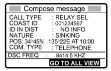
14. Press the [CALL] key, and the message "Category distress transmit sure?" appears. Continue pressing the key until the display shows "Distress relay sel call in progress!" to send the distress relay call.
