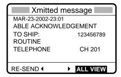
4. Press the [CANCEL] key. You can now communicate with the party, over the radiotelephone frequency specified or by the NBDP terminal unit.
