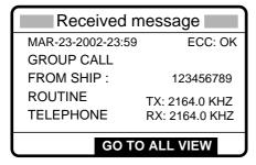
3. Press the [CANCEL] key to go to the radiotelephone screen. Watch on the working frequency.
