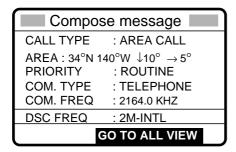
14. Press the [CALL] key to send the geographical area call (transmission time: about seven seconds). The display shows "Geographical area call in progress!" while the call is being sent.
