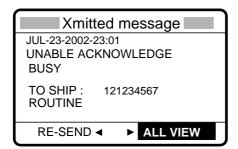
4. Push the [ENTER] knob to confirm the message. Rotate the [ENTER] knob to scroll the message. Choose GO TO EASY VIEW and then push the [ENTER] knob.
