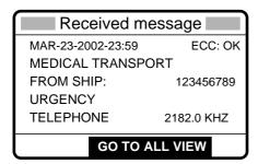
3. Press the [CANCEL] key to go to the radiotelephone screen to watch on frequency specified.
