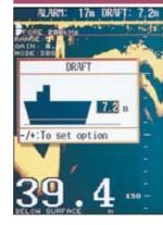
Depth Below Surface mode provides a draft-adjusted depth reading and is useful in referencing to the nautical chart. The draft is adjustable with the [DRAFT] key at the DBS position of the Mode Selector. If you find any difficulty to check for the draft value, use the NAV mode, where vou can find the bottom clearance under the keel.
